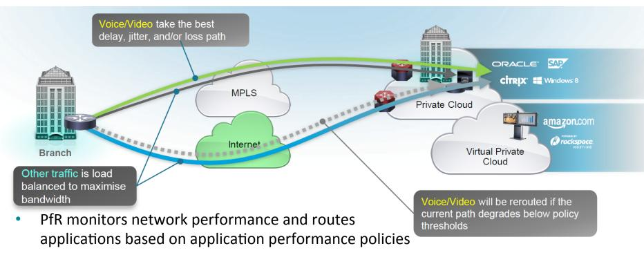
PfR load balances traffic based upon link utilization levels to efficiently utilize all available WAN bandwidth
